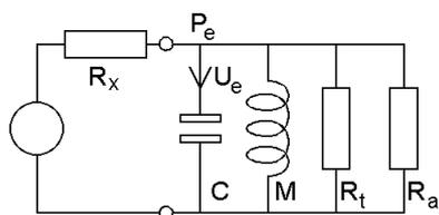
Figure 3: A resonator modeled as a single RMC parallel circuit, with resonance angular frequency  $\omega=(MC)^{-1/2}$  and quality factor  $Q=R/(\omega M)=\omega C/R$ , where R is the parallel combination of exciter, turbulence and acoustic components.
