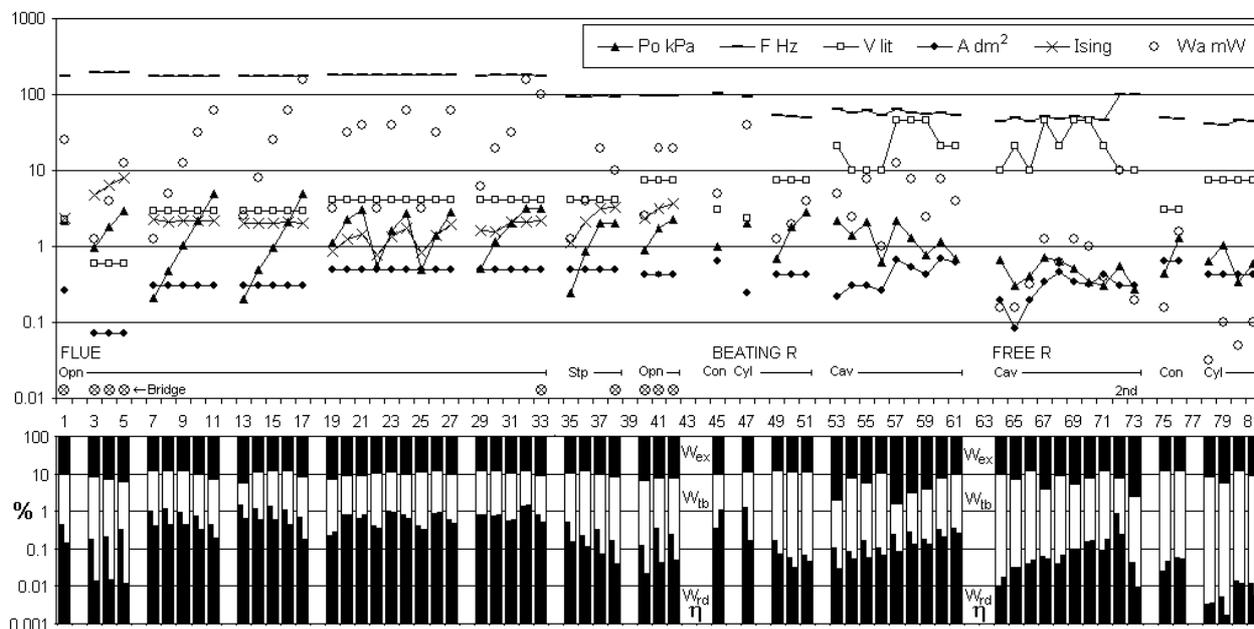
Figure 1: Top: Some dimensional data and measurements for the pipe samples. Bottom: Computed cumulative percentage of input power developed in radiated sound  $W_{rb}$ , resonator loss  $W_{tb}$ , and the excitation mechanism  $W_{ex}$ .  $W_{rd}$  corresponds to efficiency  $\eta$  and is split into a left bar for the result found from external sound, and a right from internal sound pressure.
