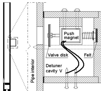
Figure 6: Cavity detuner at a flow node.
